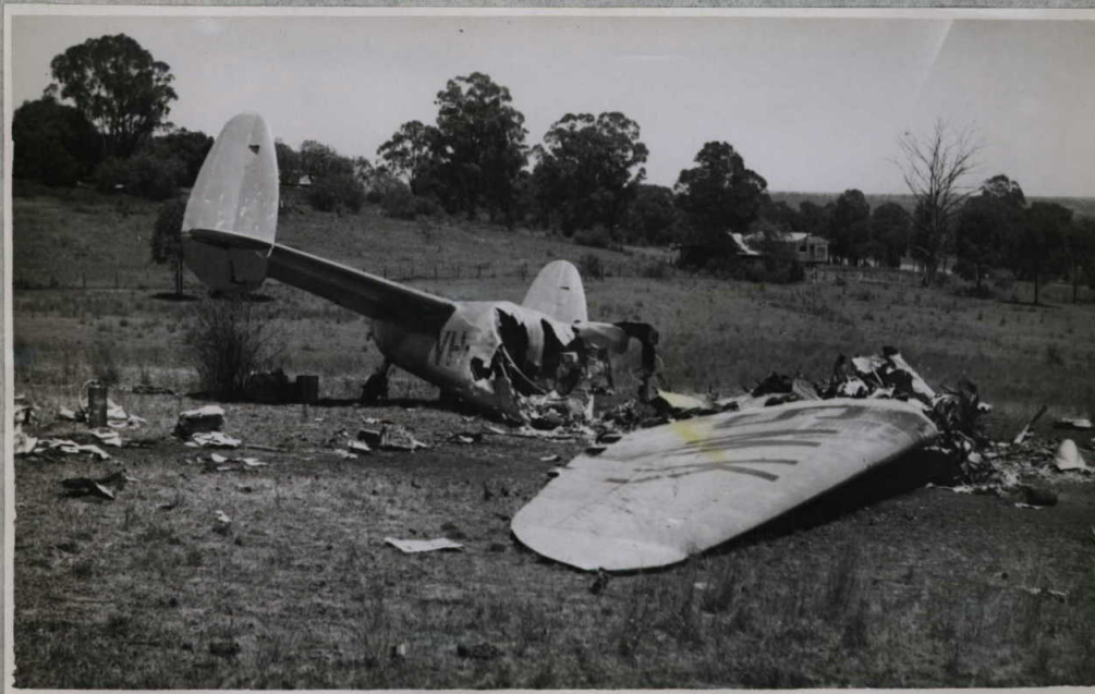
3. Relationship of starboard wing to fuselage.
