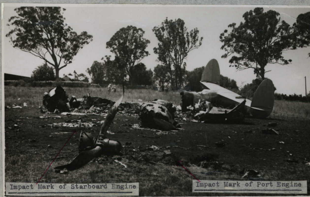
2. General view showing extent of fuselage damage, initial impact marks of both engines, and general movement of wreckage to starboard and to the rear.
