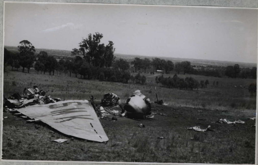
6. Damage to starboard wing at trailing edge of outer section and showing position of starboard engine.
