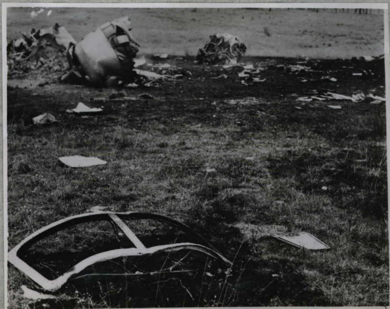
16. Escape hatch relative to main wreckage.
