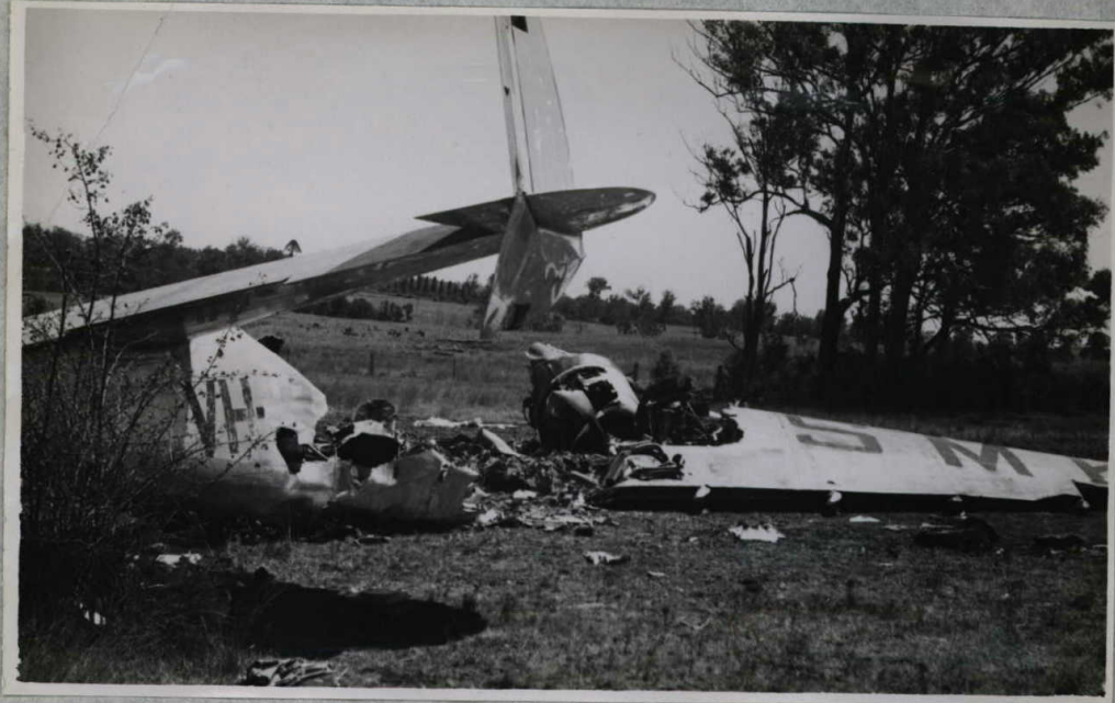
5. Damage to starboard fin and rudder
