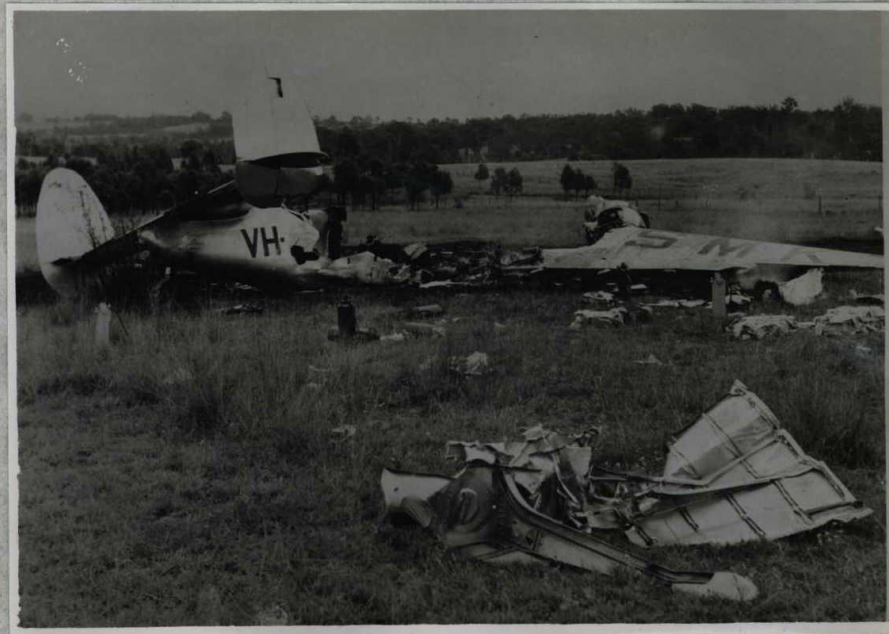
7. Position of portion of port wing relative to wreckage.
