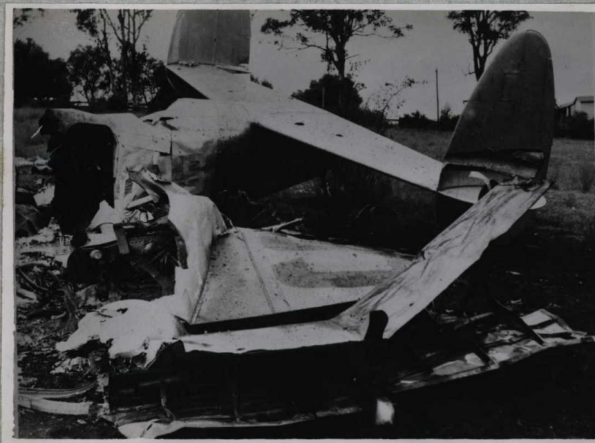
4. Only substantial portion of port wing remaining, consisting of approximately 5 feet outboard of and including wheel well, lying inverted.
