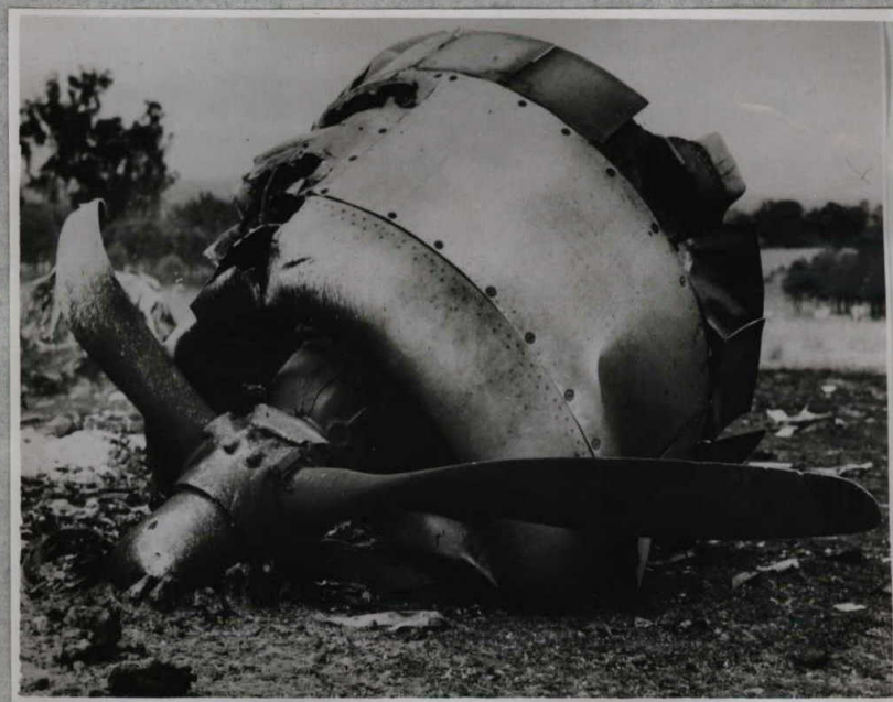
10. Starboard engine, one airscrew blade bent to rear and burnt, second blade showing only superficial damage.
