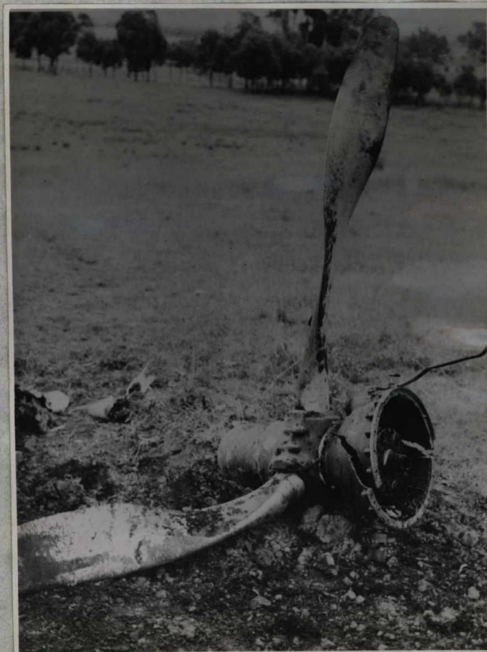
12. Port airscrew and reduction gear cover detached from engine on impact showing nature of blade damage.
