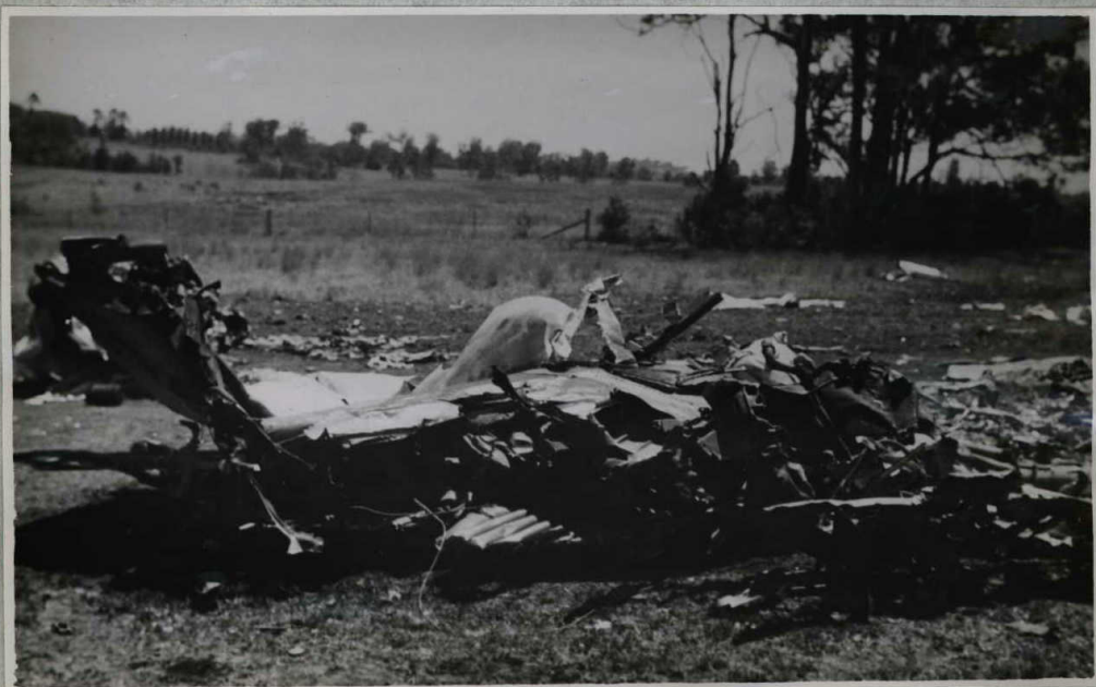
8. Remains of port mainplane viewed from tail of the aircraft, leading edge faces camera.
