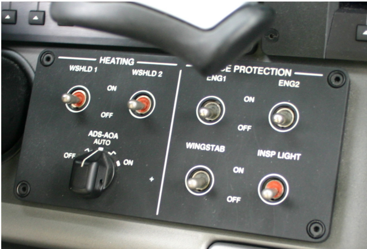
Abb. 2: Bedienpanel Ice Protection/Heating
