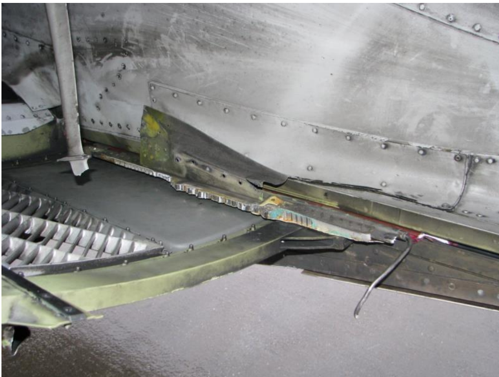
Image 4: Remnant of the torn off fan reverser translating cowl stuck in the rail
