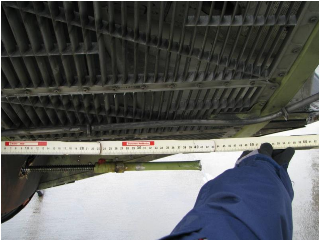
Image 3: Extended and fractured ball screw shaft
