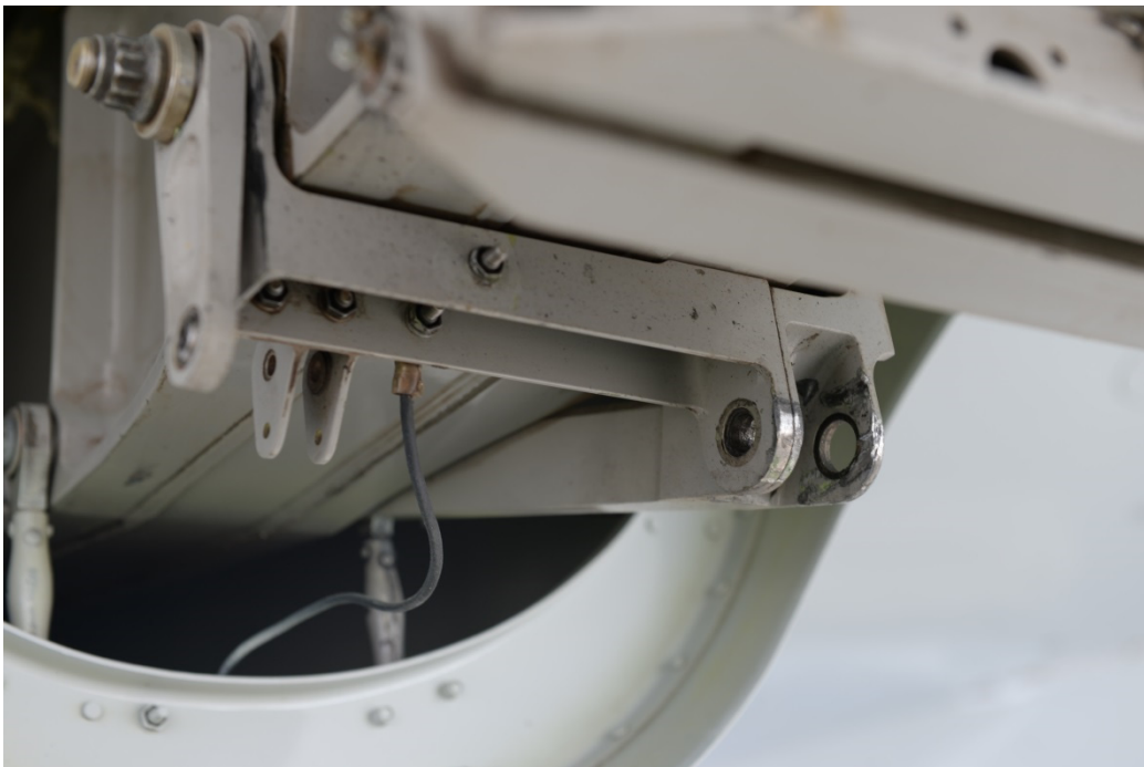
Image 4: Front mounting points on the flap track and carriage
