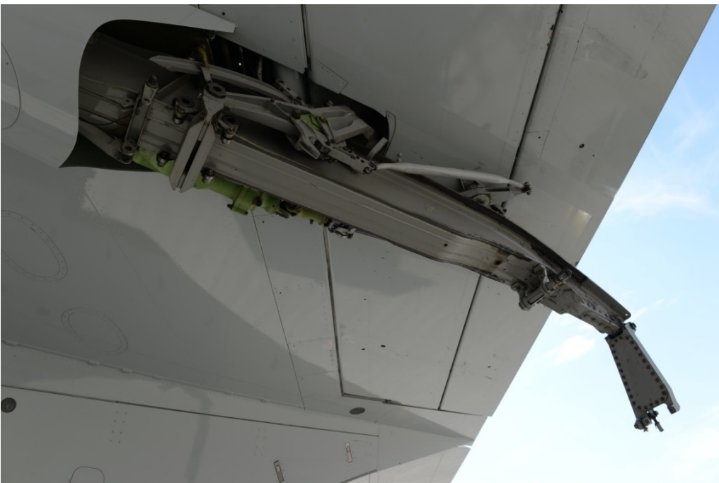
Image 2: Outer flap drive and flap track and carriage on the right wing
