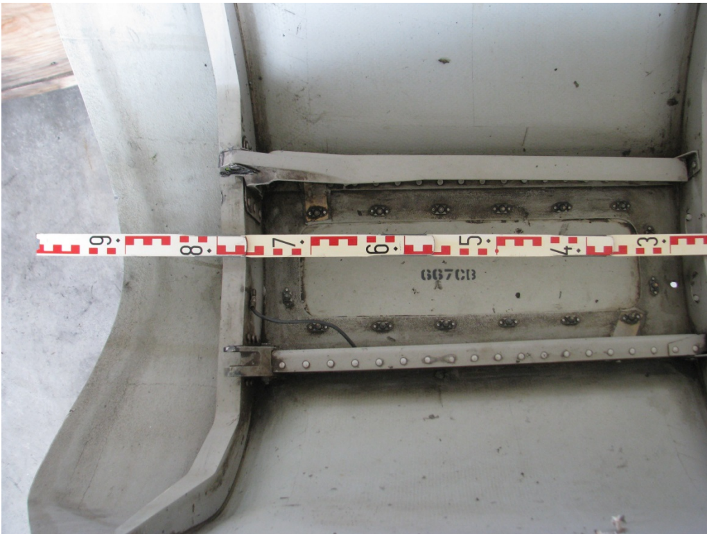
Image 5: Front mounting points on the fairing
