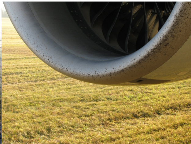
Dirt on the right engine
