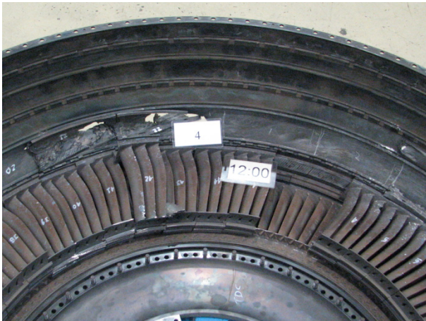
The 4th stage stator stage with two missing vane clusters
