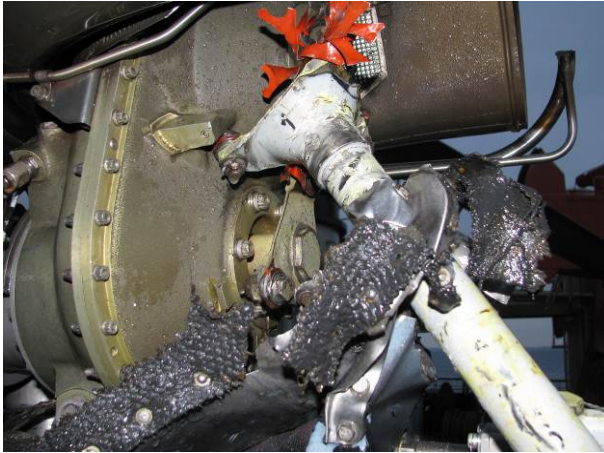
Damages on the forward coupling of the tail rotor drive shaft
