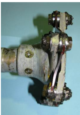
Damages on the rear coupling
