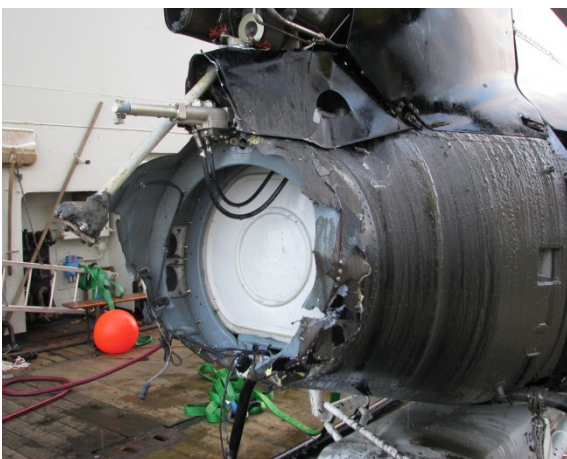
Damages on the aft fuselage and the Star-Flex
