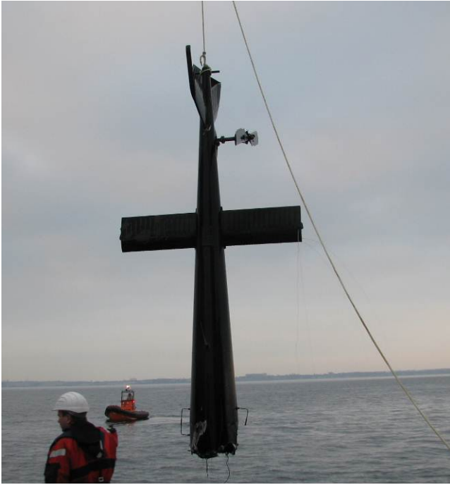
Damages on the forward tail rotor drive shaft fairing and coupling
