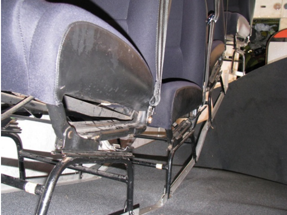
Damages of the mountings of the third, fourth and fifth right seats
