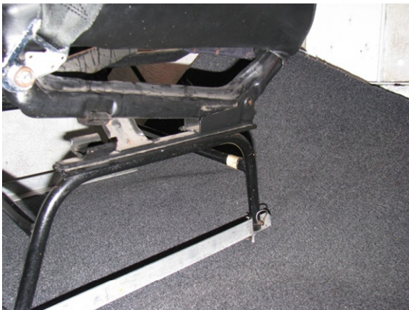
Damages on the mounting of the first left seat
