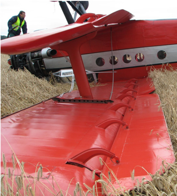
Damages on the wing structure and position of the flaps
