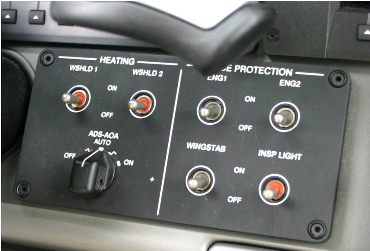
Panel of the ice and rain protection system
