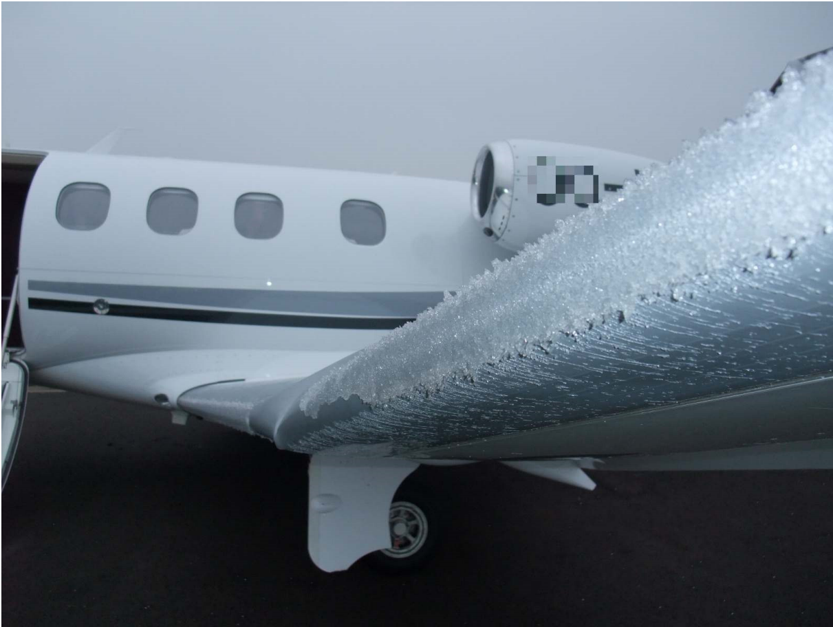
Ice accretion on the left wing leading edge
