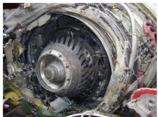
Right engine had been running at high speed
