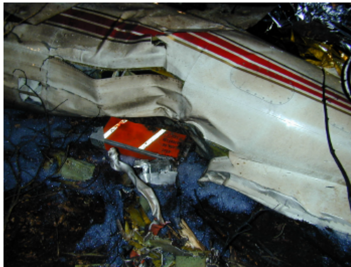
Tail Section and Flight Data Recorder
