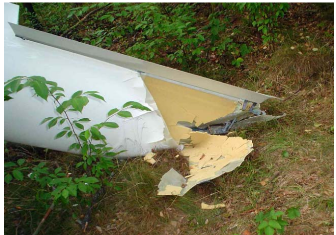
Picture 3: Left wing's point of rupture
