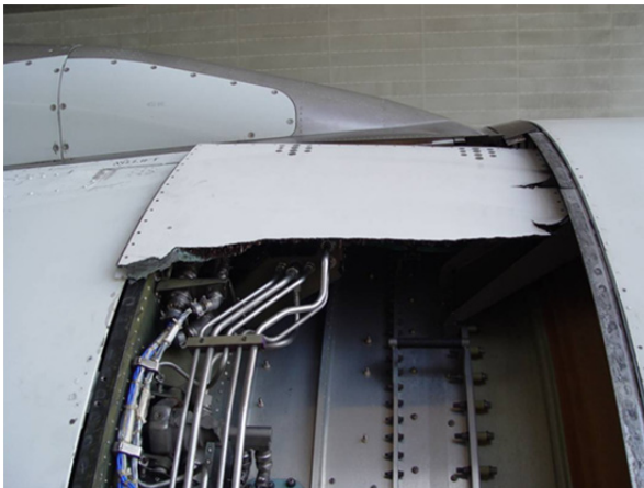
Residual fracture, right and left side
