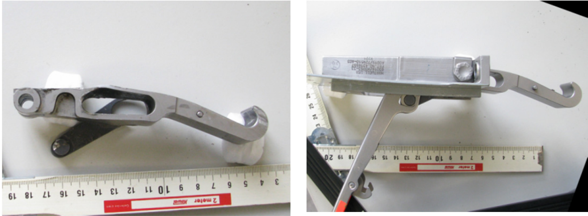
The approximate position of the link versus an undamaged latch
