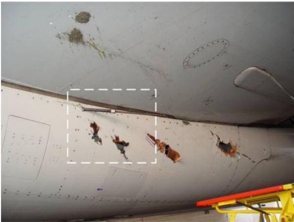
Damages to the belly fairing
