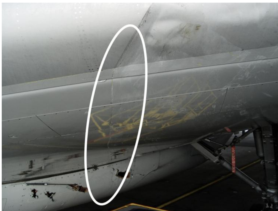
Continuous scratch mark on the lower surface of the wing
