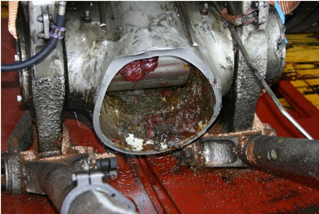
Image 2: Front part of the bogie beam including pivot pin
