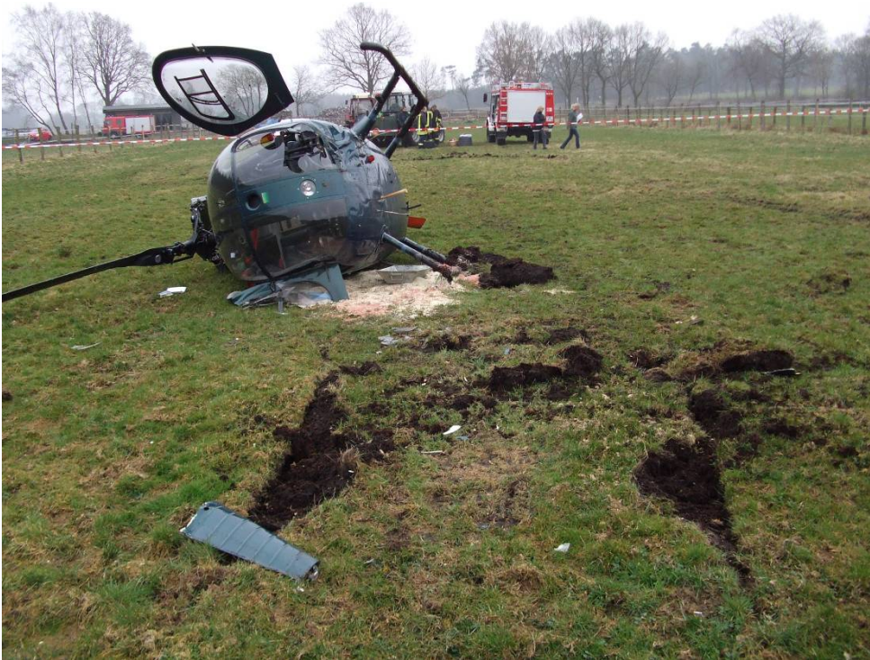
Indentation marks of the skids and wreckage position from flight direction
