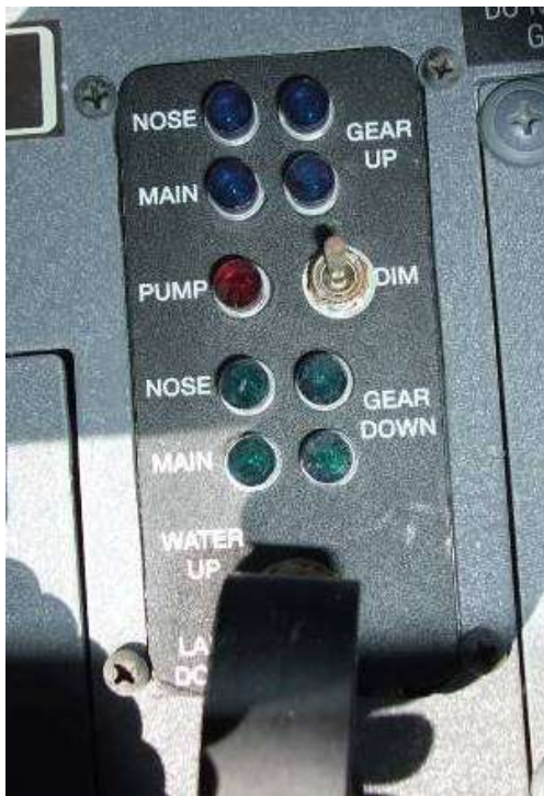
Electrical landing gear indicator in the cockpit and mechanical landing gear indicator on the floats
