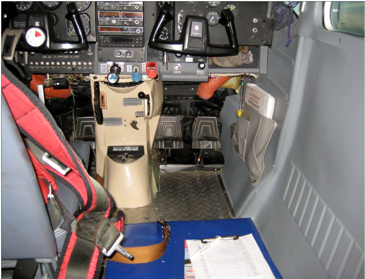
Cabin of the Cessna on the day of the accident, missing co-pilot's seat
