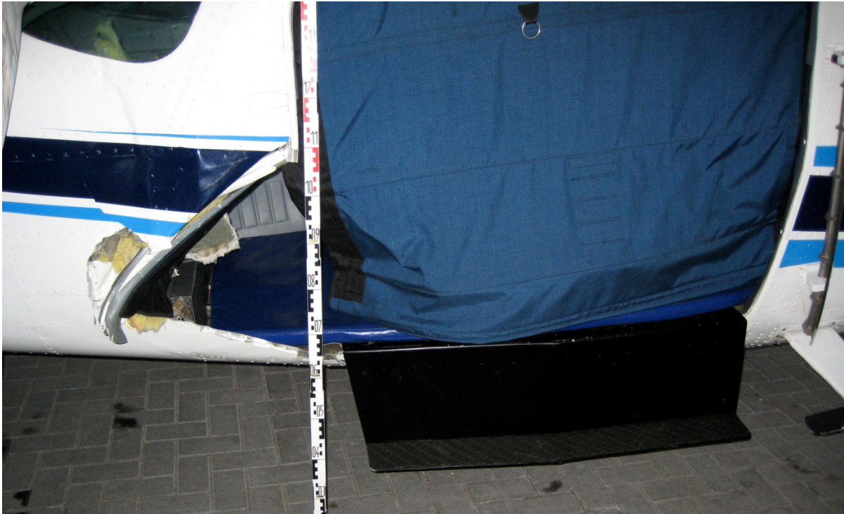
Closed door and damages in the area of the door
