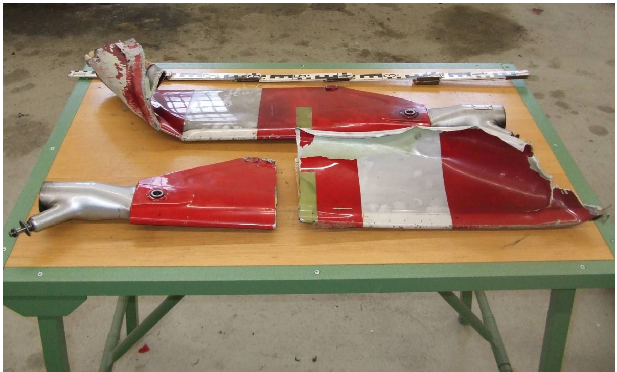
Appendix 2: Damage to the helicopter's tail and tail rotor blades
