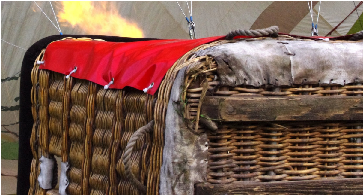
Visibly fractured basketwork on the bottom (prior to take-off / rigging process)
