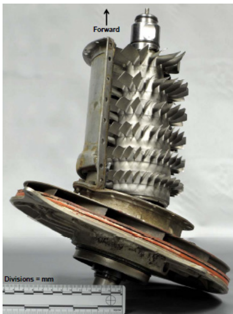
Compressor with blades bent against the normal direction of rotation
