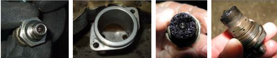
Detailed photos: chip warning detector; fuel filter housing; fuel injection jet Photos: BFU
