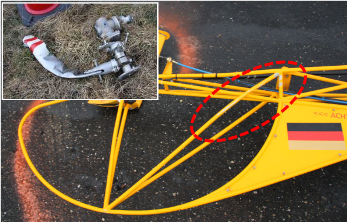
Tail rotor gear box including tail rotor blade and damages on the tail boom
