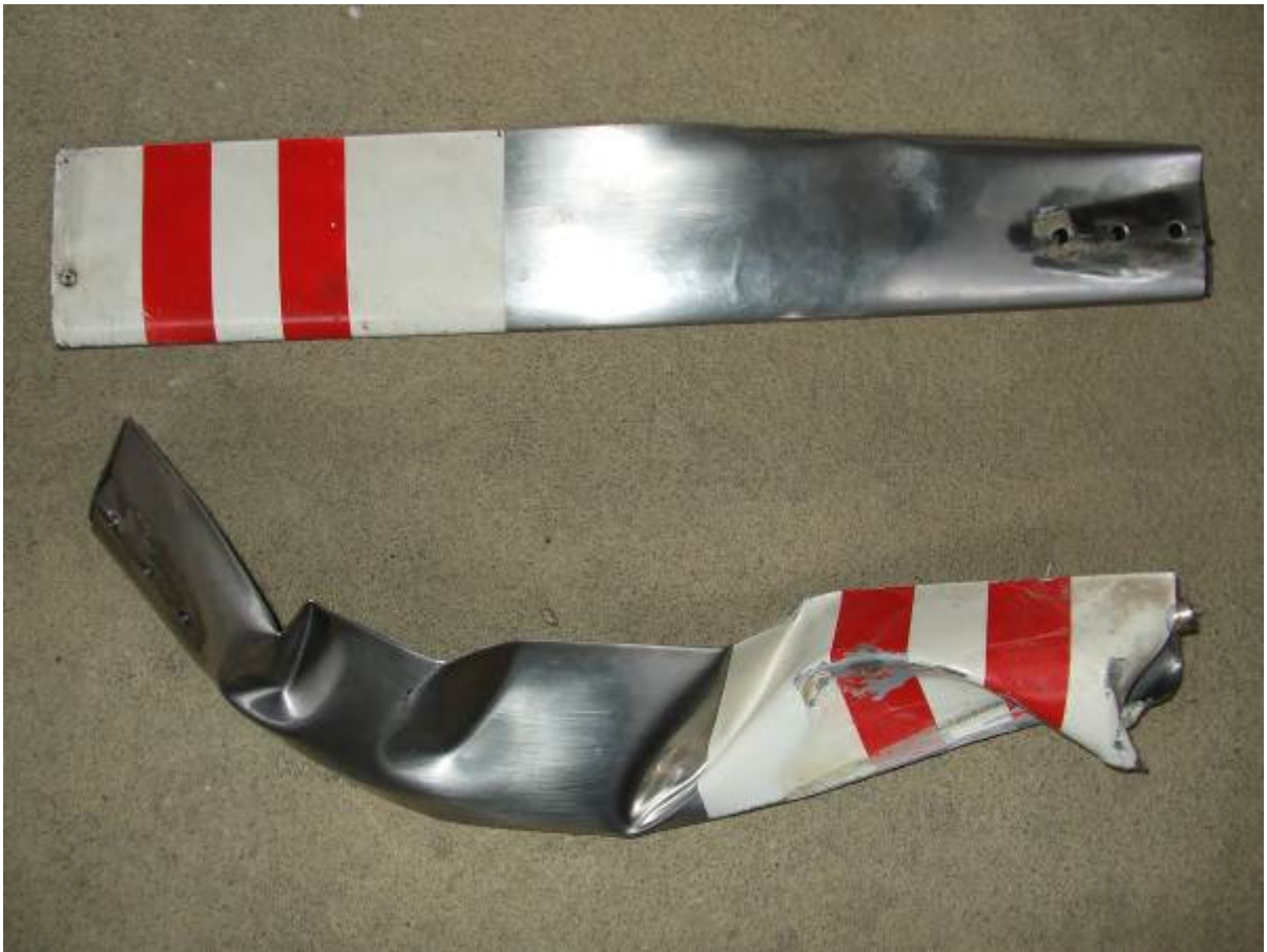
Fractured tail rotor spindle and the two tail rotor blades
