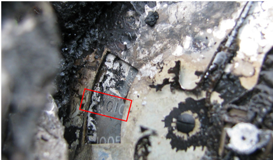
QNH selection at the altimeter about 1,010 hPa
