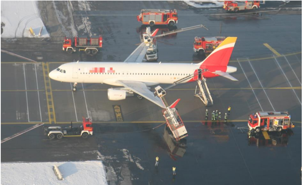
Positions of the airplane and the de-icing vehicles after the collision
