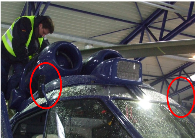
Mirror for the inspection of ice accretion on the closed MPAIs
