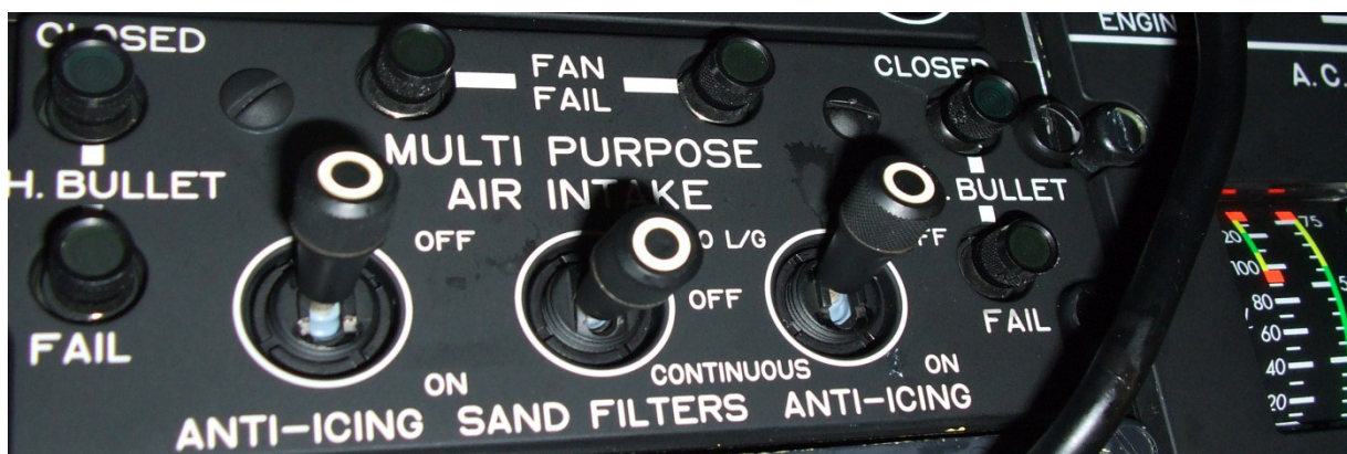
Switch for the control and function indication of the MPAs
