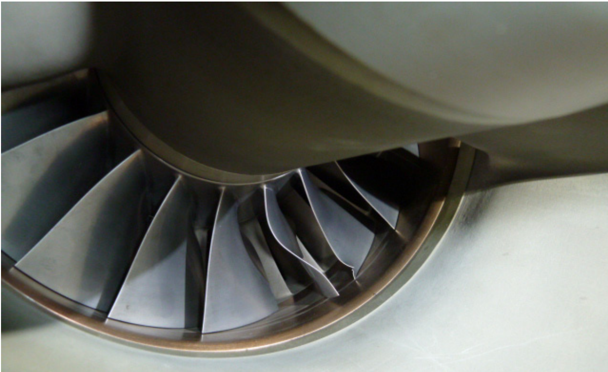
Damage on the compressor of the right engine
