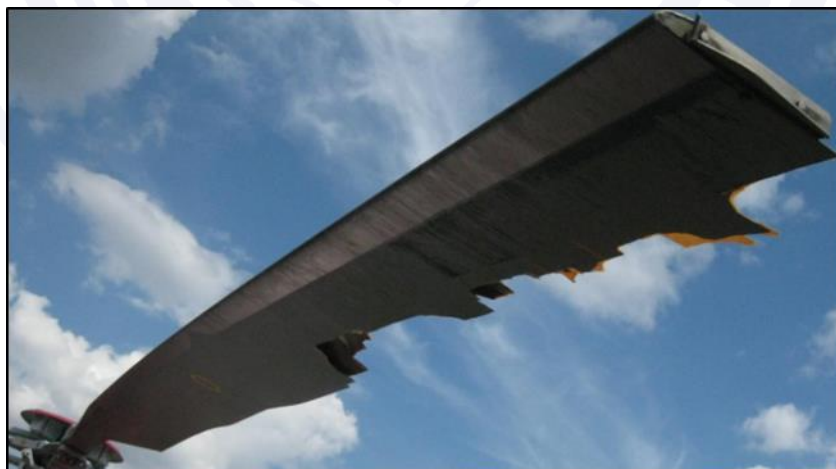
Figure 3 - Extension of damage to the main rotor blade.
