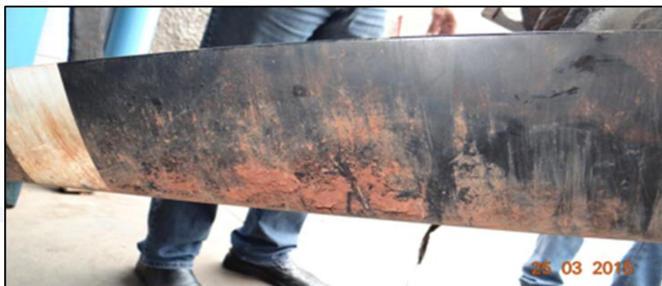
Figure 3 - View of the propeller with dirt deposited along the blades.
