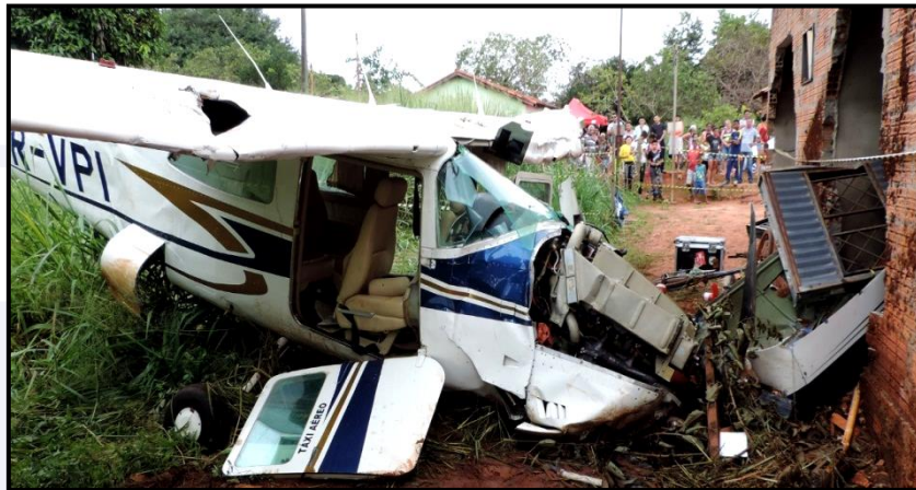
Figure 4 - Damage to the front section and the wings.
