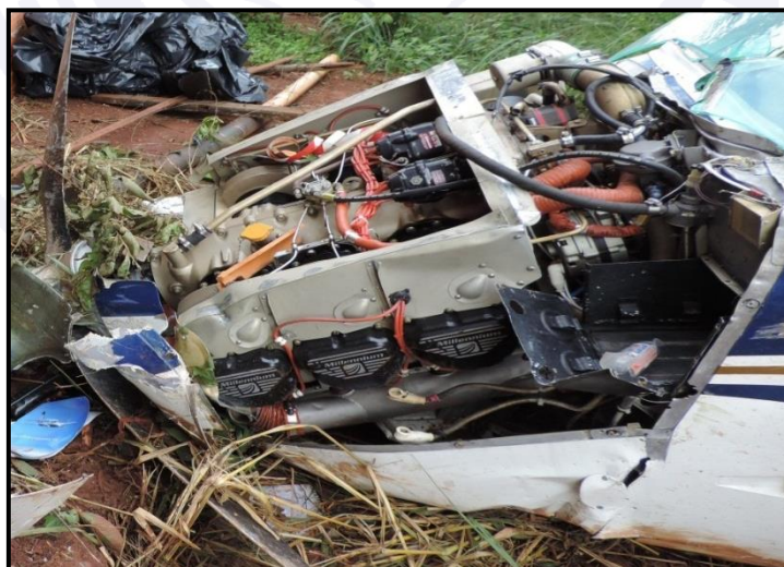
Figure 6 - Situation of the engine after impact.
