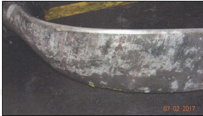
Figure 8 - View of the blade with the transversal scratches.
