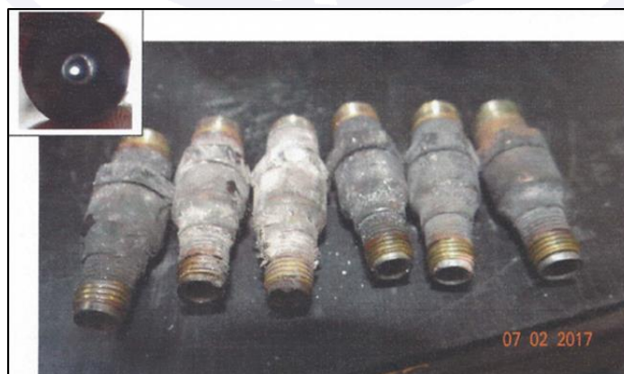
Figure 7 - View of the engine nozzles. Highlighting one of the unobstructed nozzles.
