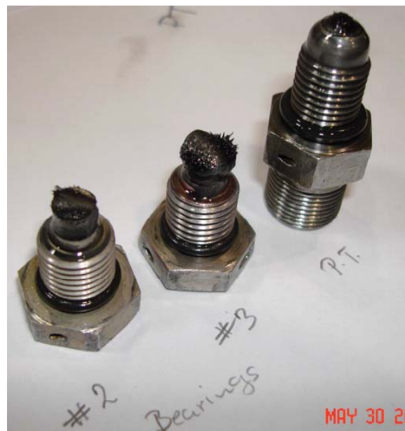
Magnetic plugs for main bearing number two and three and power turbine.
