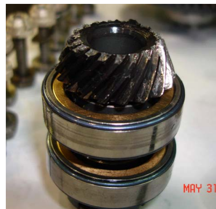
ADG bevel pinion assembly, bearings and teeth.
