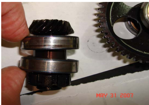
ADG bevel pinion assembly, bearings and teeth.
