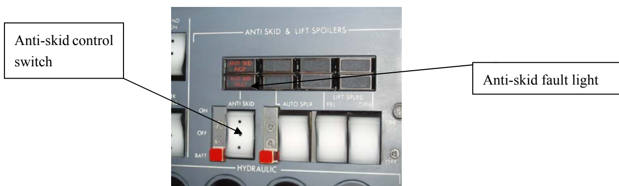
Anti-skid control panel
