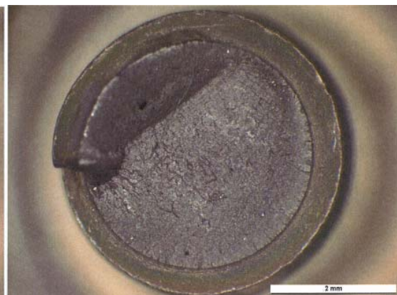
Photo no. 3 The fracture surface of bolt B.
