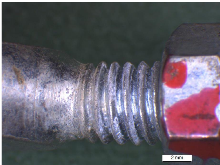
Figure 10 Forward right hand steering rod threaded rod end, free of fracture marks and corrosion.
