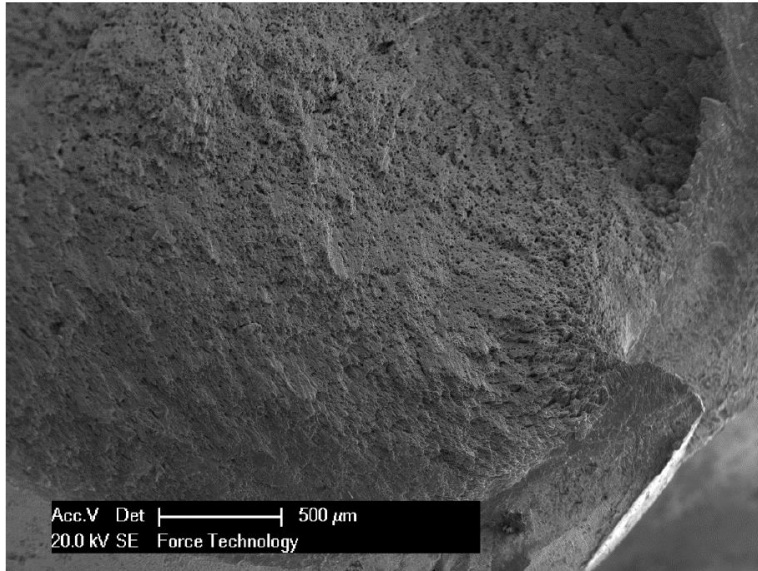
Figure 17 SEM micrograph of aft left hand steering rod fracture surface.
