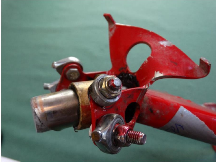
Figure 3 Main steering frame with significant signs of deformation.
