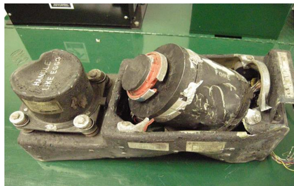
Figure 3- Tarsyn – 333 Three Axis Reference P/N: 2593996-333, S/N 0050220
