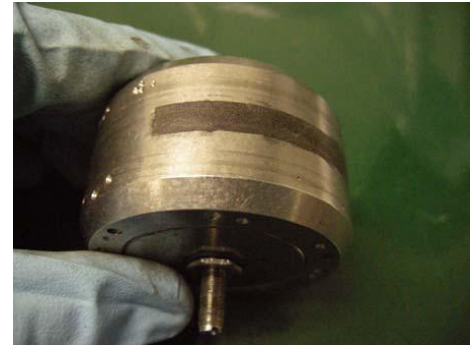
Figure 5- Gyro rotor surface P/N: 2593691 S/N: 6093099 fitted to Tarsyn – 333 Three Axis Reference P/N 2593996-333, S/N: 6093099
