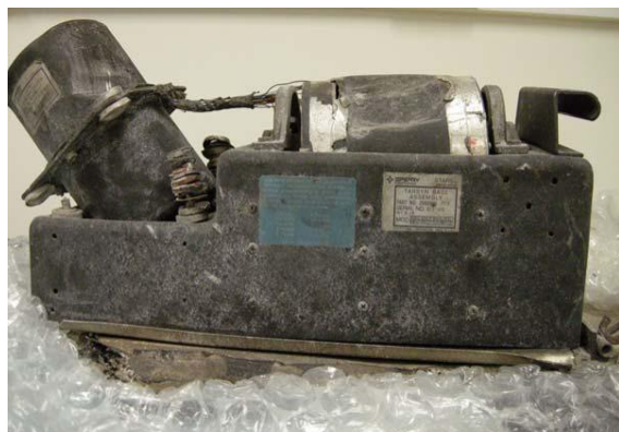
Figure 2- Tarsyn – 333 Three Axis Reference P/N 2593996-333, S/N: 6093099
