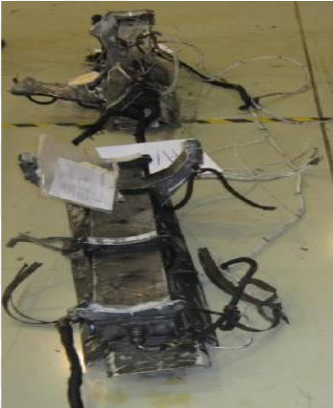
Photo 31. Recovered junction boxes from A6EMR. 5
