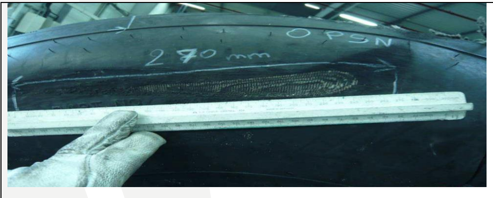
Photo 17. Opposite serial Number friction cut, Tire Position 5.
