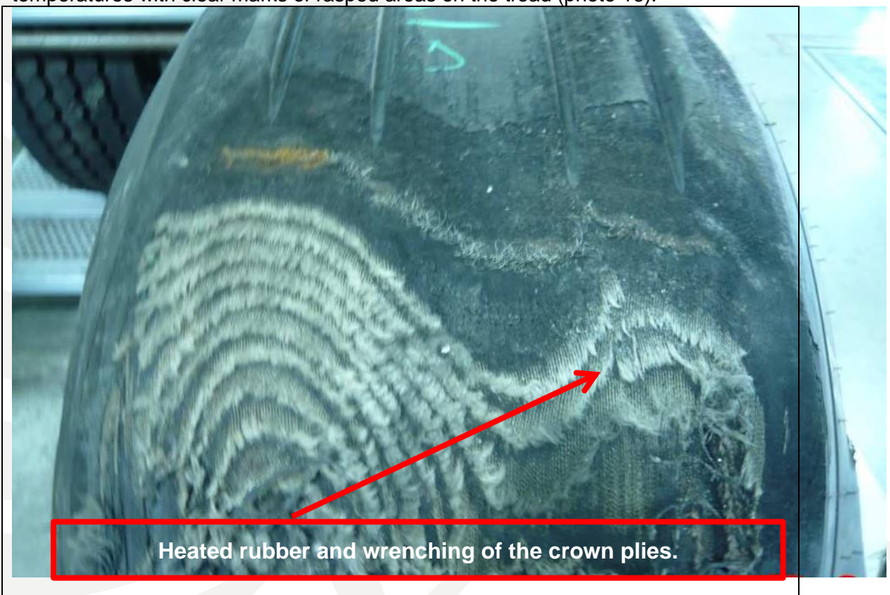
Photo 16. Flat Spot heated rubber, Tire Position 5.
