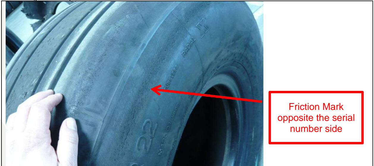
Photo 23. Opposite serial number sidewall friction mark, Tire Position 6.
