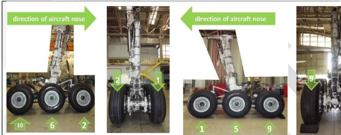
Figure 2. B777 (left) landing gear
