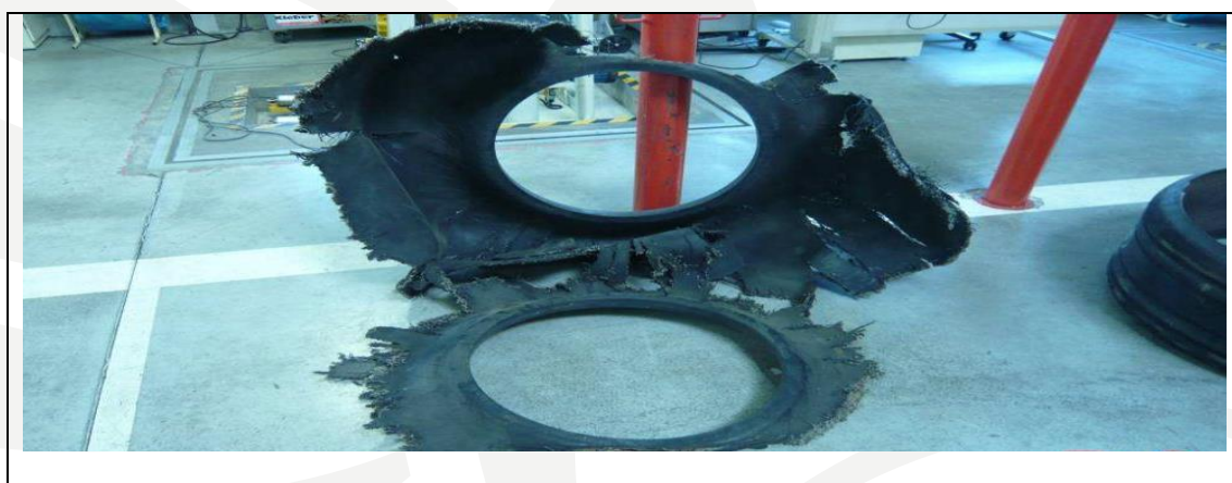
Photo 14. Total dislocation, Tire position 2.
