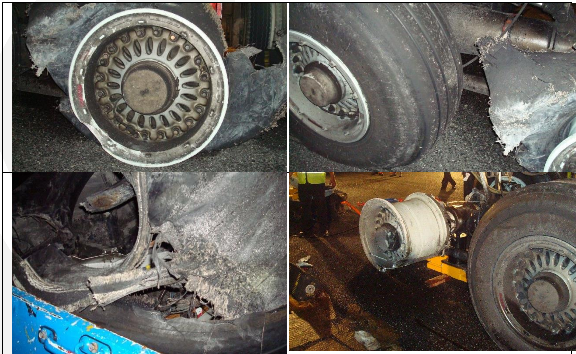
Figure 1. Photos indicating the condition of the landing gears' hubs and tires at Male airport prior to removal from the aircraft.
