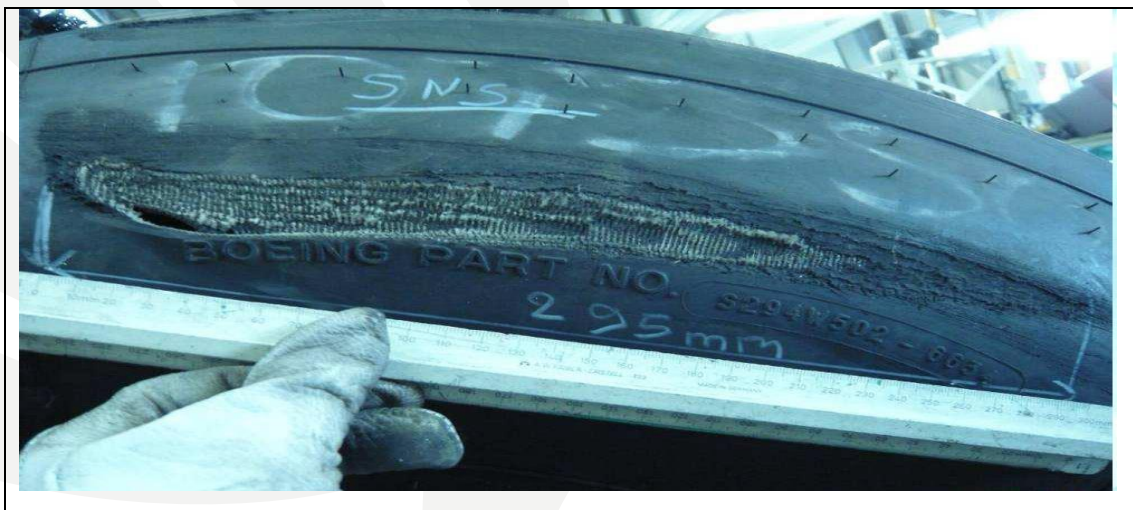
Photo 18 Sidewall on the serial number side friction cut, Tire Position 5.
