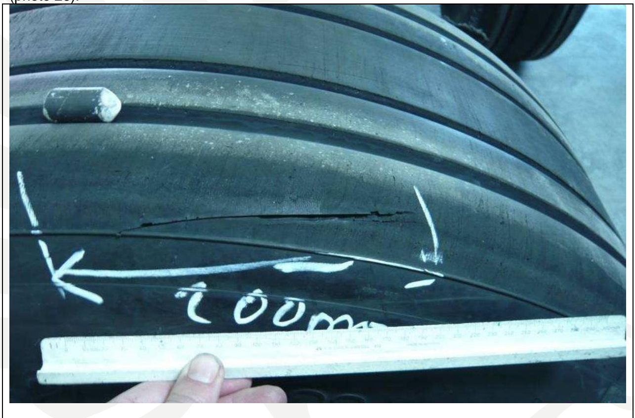
Photo 26. Shoulder cut on the opposite serial number side, tire position 9.
