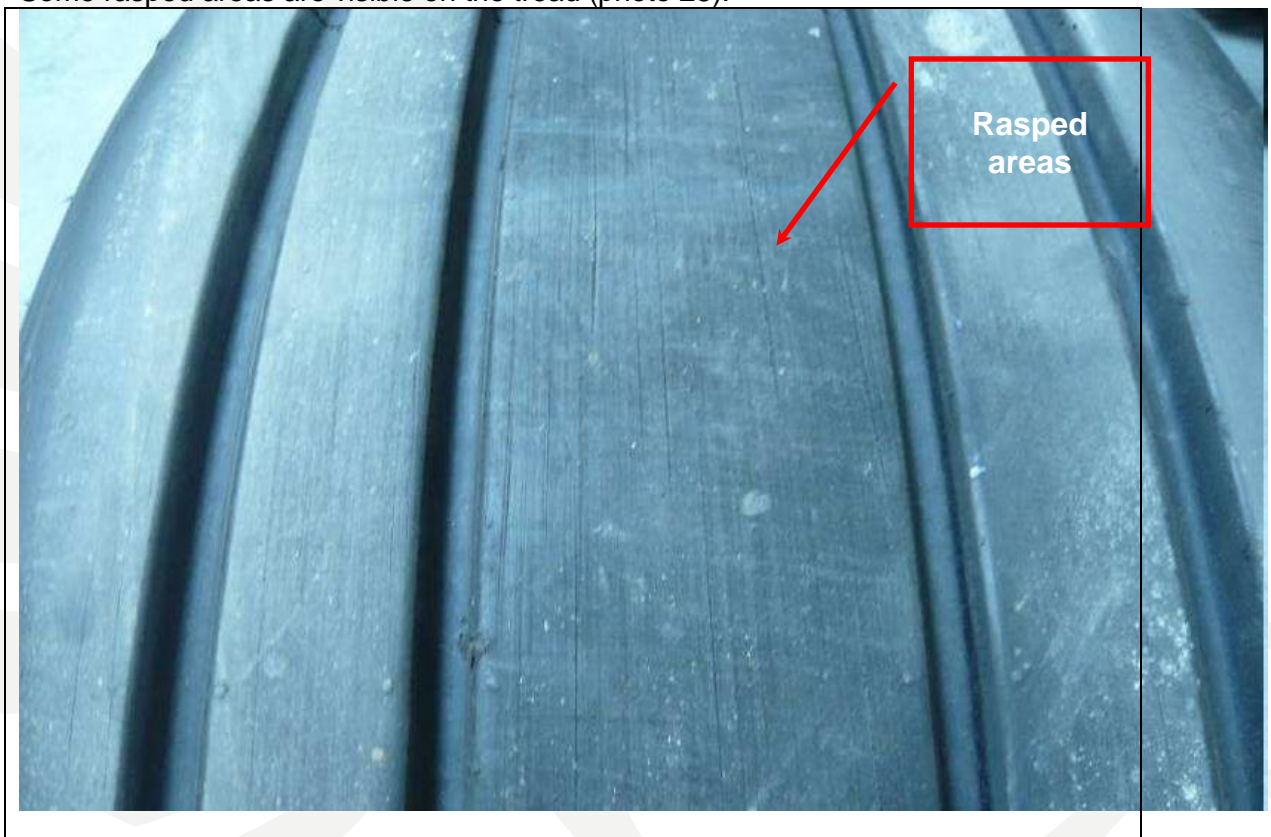
Photo 28. Rasped areas on Tire Position 10.
