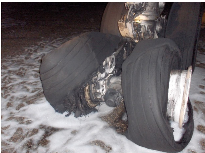
Figure 1. Condition of tires on wheels 5 and 6
