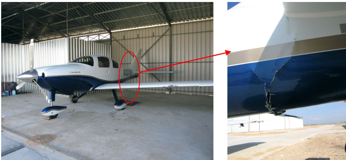
Figure 1. Close-up of the damage evident in the right wheel fairing and in the tail
