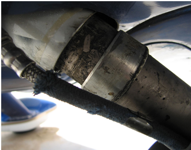
Figure 5. Close-up of the right wheel bushing displaced from its housing
