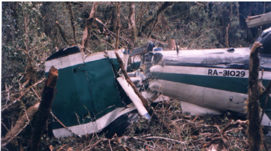
Picture 3. Static loading damage on the tail
