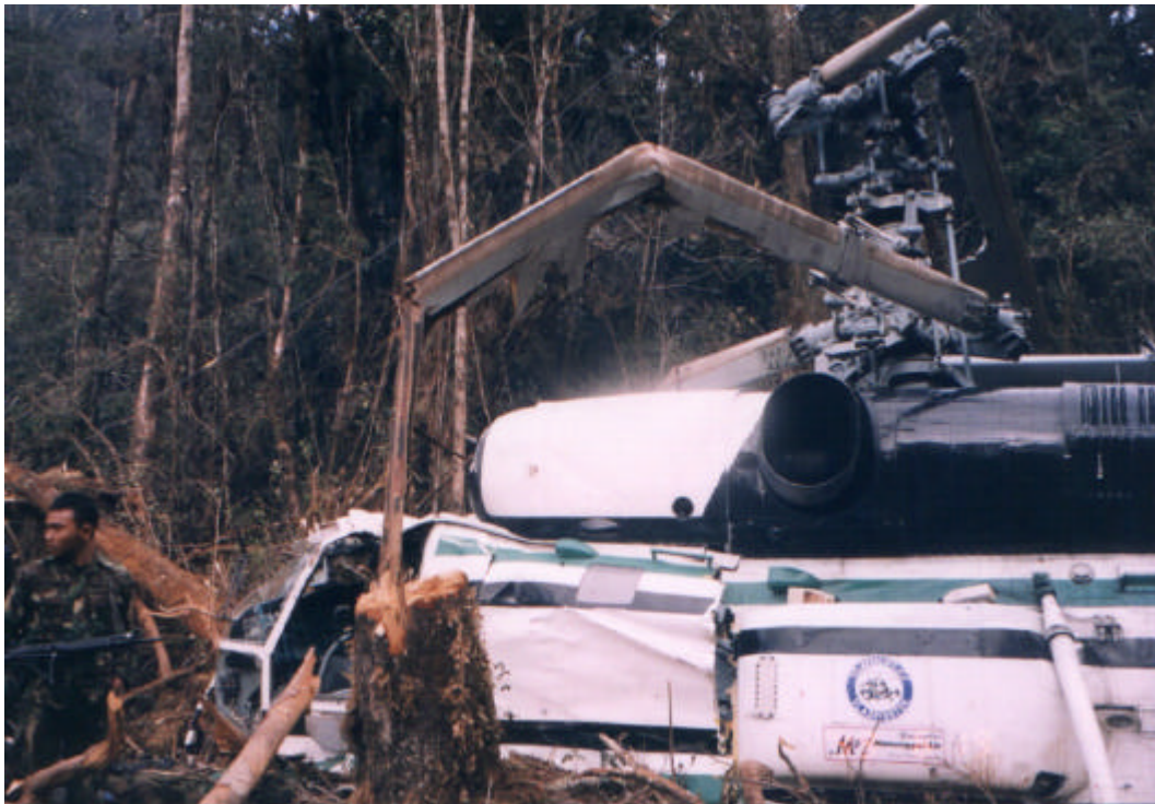
Picture 2. Damages on the rotor blades indicating rotation at impact
