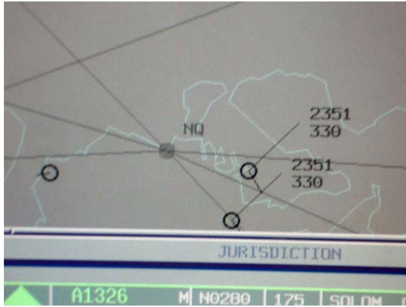
Figure 12: The aircraft at 01:06:51, was still at FL 330 (altitude 33,000 feet) and captured by two radar heads
