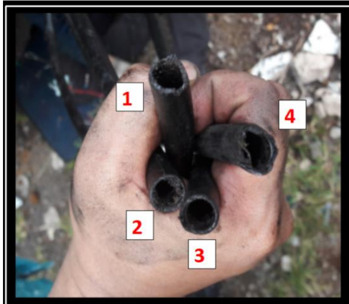
Gambar 13. Selang service cylinder brake patah.
