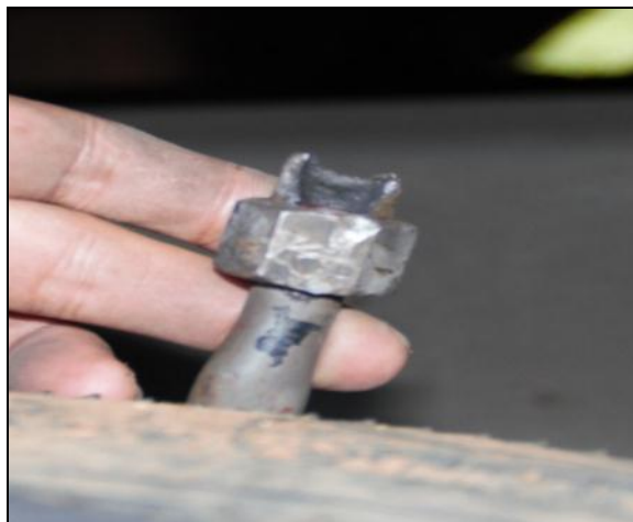
Gambar 14. Selang udara front brake chamber patah
