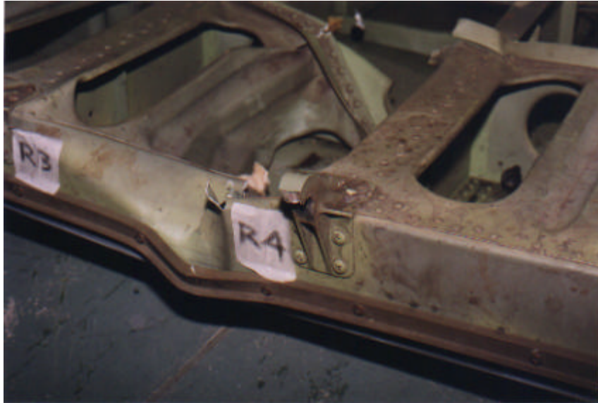
Photograph 2. Broken Guide Hook (R4)
