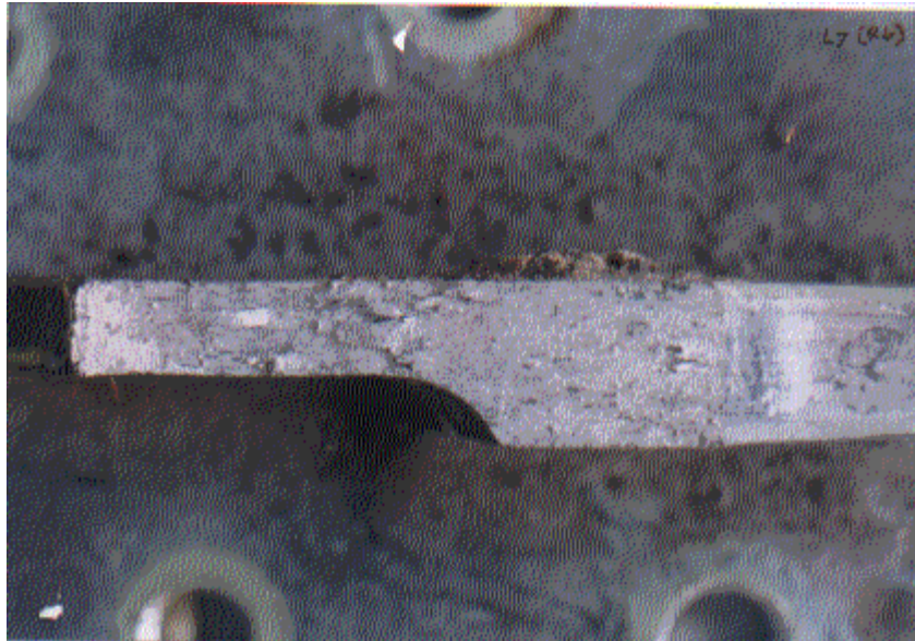
Photograph 7. Macroscopic Photograph on L7 Port Fitting Fracture Surface
