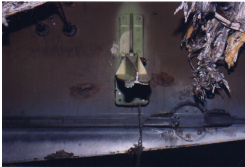
Photograph 3. Broken Hinge and Half Hinge Assembly
