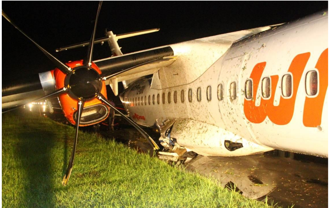
Figure 2: The damaged main landing gear and propeller
