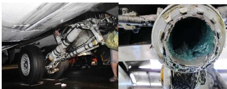
Figure 2: The collapse left MLG and broken trunnion link
