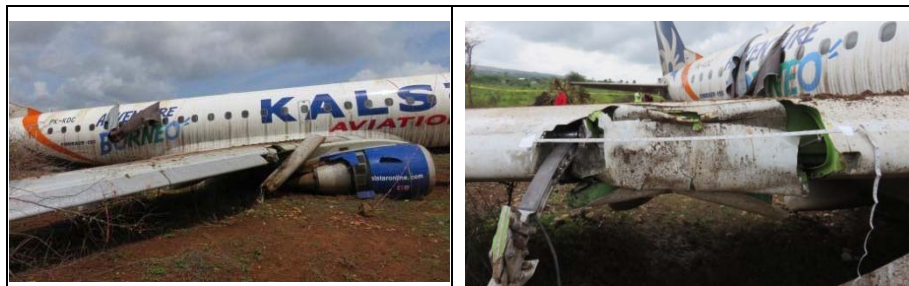
Figure 1: The damaged right wing
