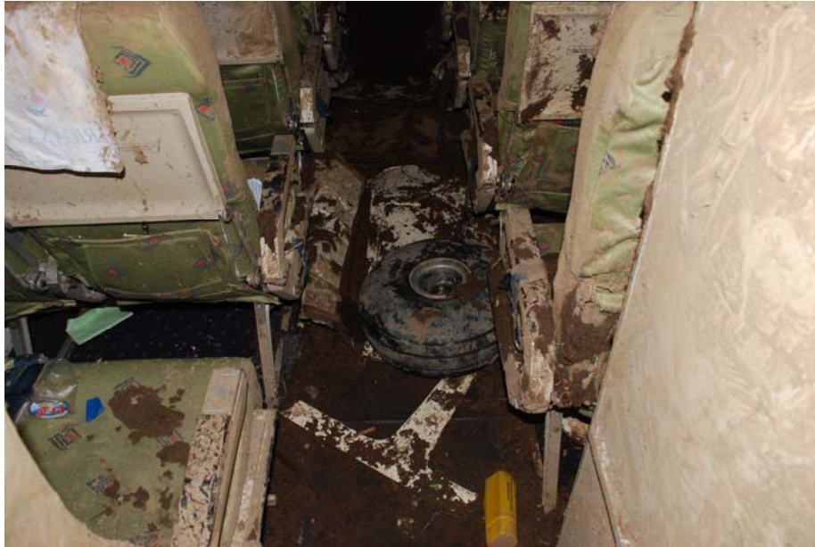
Figure 8: Nose wheel found inside the cabin
