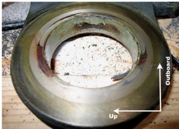
Figure 8 Wear/corrosion deposits on wear face of the intact inner washer on the trailing side of the yoke
