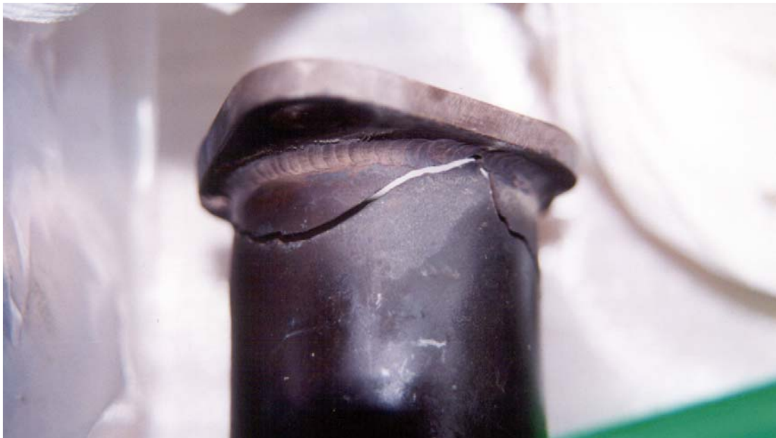
Cracked Exhaust Stub Fig. 2
