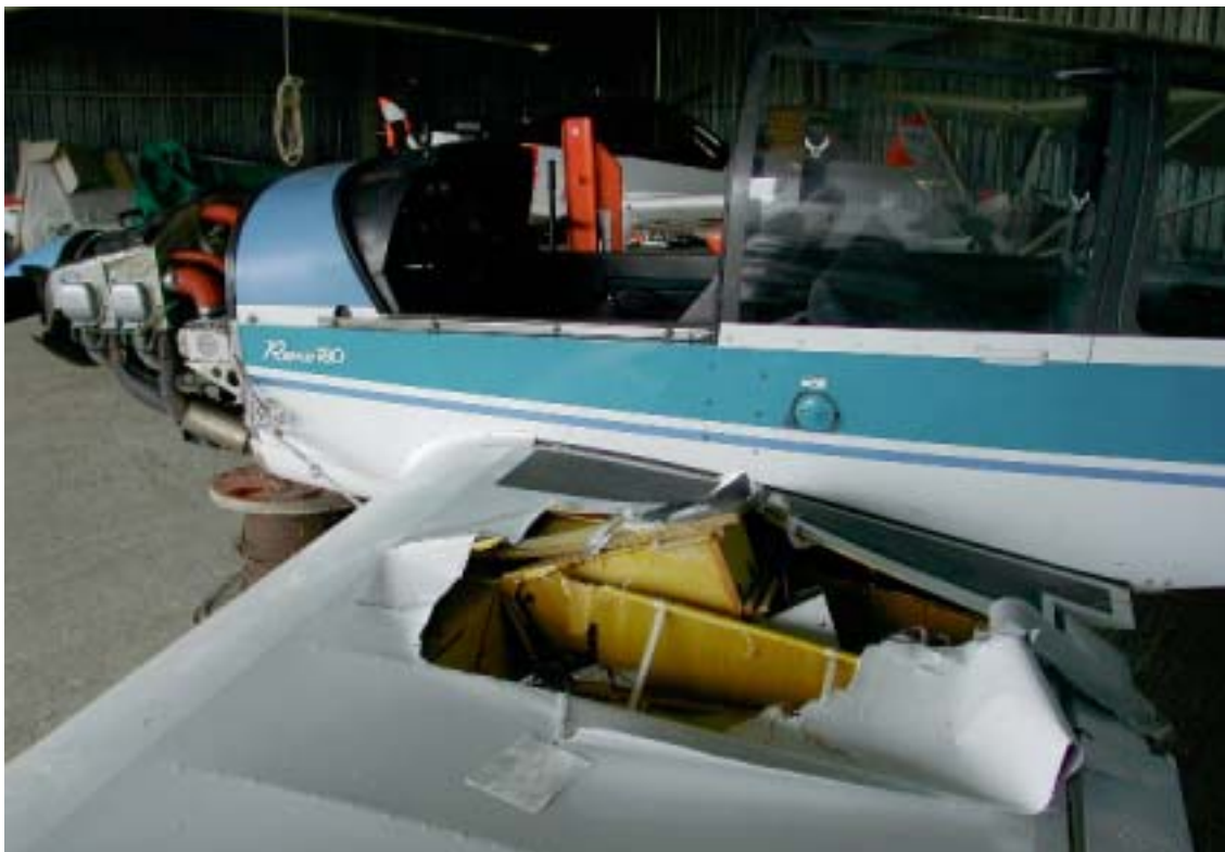
Velivolo in hangar. Danni semiala SX.
