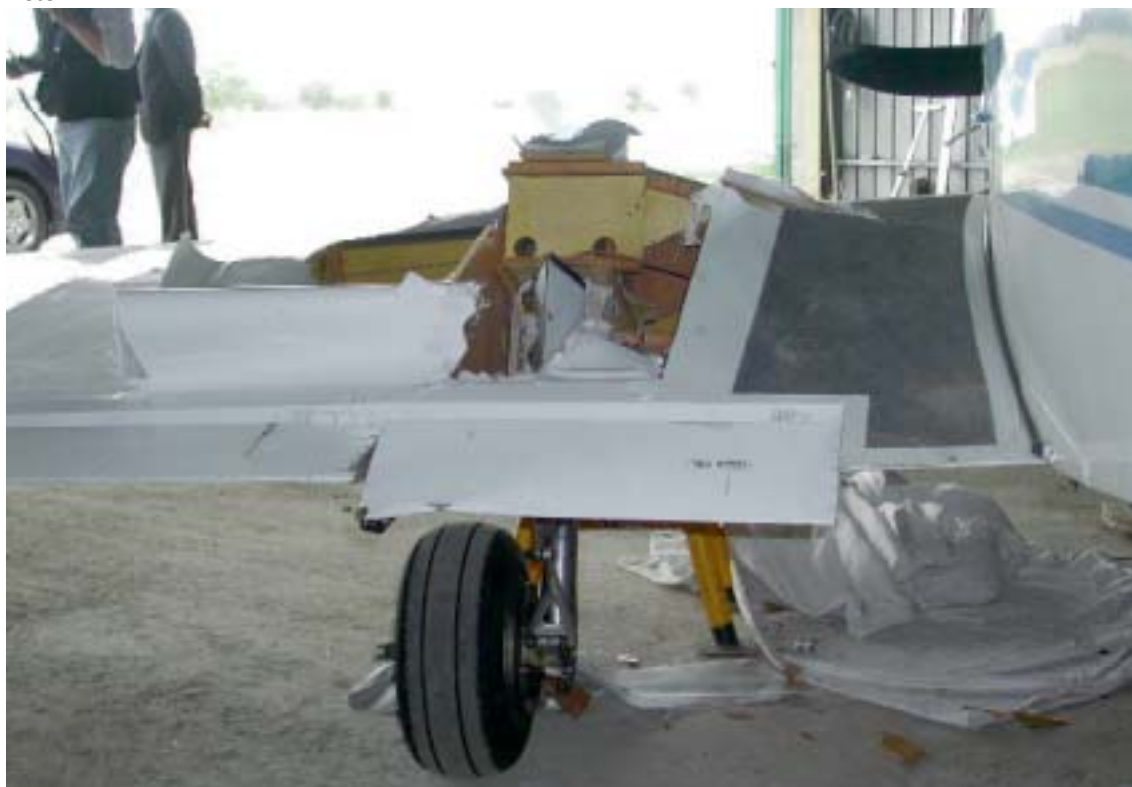
Velivolo in hangar. Semiala SX. Notare danni alettoni e flaps
