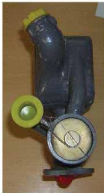
Picture 3: "oil to fuel heater".
