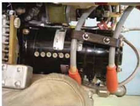
Picture 3: original APU Starter electrical connectors.
