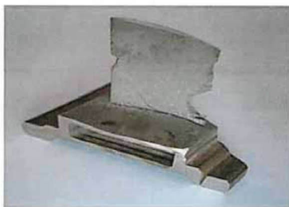
Figure 3: fragment of upper half-ring 5 th stage with vane N° 1 - external ring.
