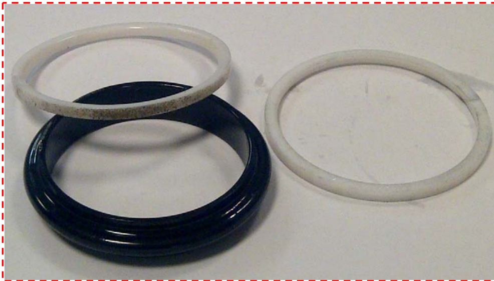
Picture 8: contamination found on LH MLG door actuator.
