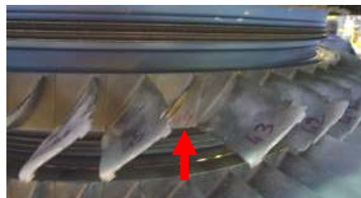
Stage 4 HPC #44 blade with airfoil missing, (separated just above the platform).
