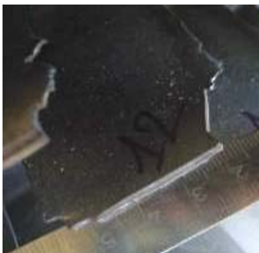
Stage 4 HPC: • Four of the blades (#12 shown) were found with tip corner loss on trailing edge (left hand photo); • Blade #10 found with tip corner loss on leading edge (right hand photo).
