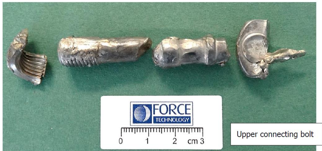
Figure 1 Parts from the upper connecting rod bolt and matching spiral lock nut after cleaning.
