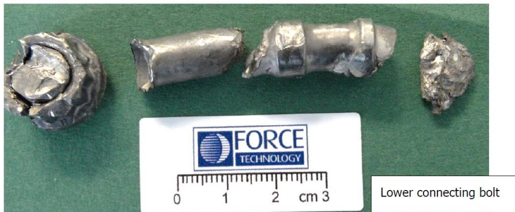
Figure 4 Parts from the lower connecting rod bolt and matching spiral lock nut after cleaning.
